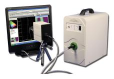
The OL 770-DMS Display Measurement System offers a complete solution for modern display measurement requirements, including R&D, production, and quality assurance, giving accurate color, luminance and spectral information instantly at the click of a button.
