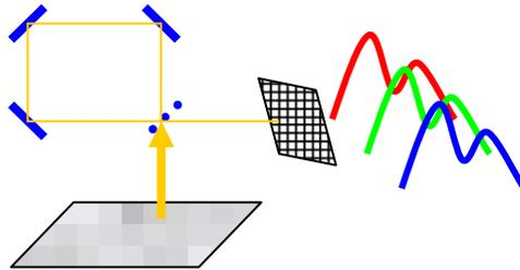
**Figure 5 - Sagnac Interferometer Hyperspectral Imager**
